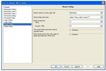
Fig. 1.8 Parameter window "Master Setting"
